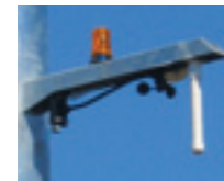
Wireless temperature receiver is attached to the spar and mounted 6.5 m up the tower.
